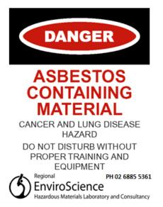
Signage should also be placed at the entry points to the building/plant similar to the one detailed
