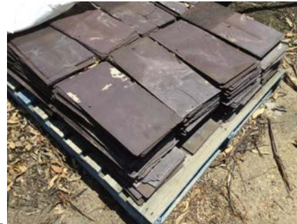
PHOTO NO.: J154900-001-PHOTO069 RESULT: ASBESTOS - NEGATIVE BUILDING/LEVEL: TRADES SHED - GROUND LEVEL ROOM/LOCATION: EXTERIOR - NORTHEAST FEATURE/MATERIAL: DUMPED MATERIAL - ROOF TILES SAMPLE NO.: J154900-001-037
