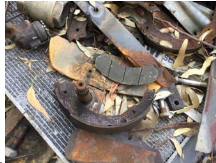
PHOTO NO.: J154900-001-PHOTO116 RESULT: ASBESTOS - NEGATIVE BUILDING/LEVEL: WORKSHOP - GROUND LEVEL ROOM/LOCATION: EXTERIOR - SOUTHEAST FEATURE/MATERIAL: DUMPED MATERIAL - BRAKE PADS SAMPLE NO.: J154900-001-046
