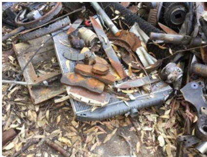
PHOTO NO.: J154900-001-PHOTO117 RESULT: ASBESTOS - NEGATIVE BUILDING/LEVEL: WORKSHOP - GROUND LEVEL ROOM/LOCATION: EXTERIOR - SOUTHEAST FEATURE/MATERIAL: DUMPED MATERIAL - BRAKE PADS SAMPLE NO.: J154900-001-046
