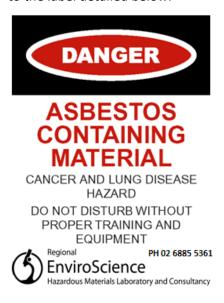
Signage should also be placed at the entry points to the building/plant similar to the one detailed below
